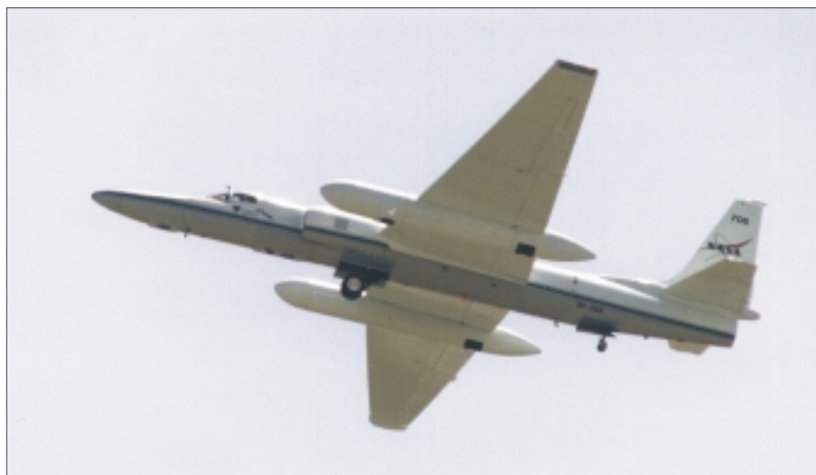
NASA ER-2 taking off. Radiation sensors for the AIR measurements were carried in the nose, the fuselage behind the cockpit, and the front third of both wing pods. (Source: DOE Environmental Measurements Laboratory, presented at the 1998 NCRP Annual Meeting, “Cosmic Radiation Exposure of Airline Crews, Passengers, and Astronauts”)
