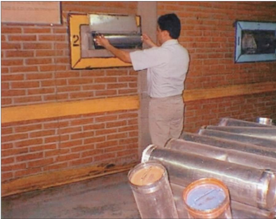
A worker at the Tuxtla Gutierrez plant loading cylinders filled with pupae into irradiators
